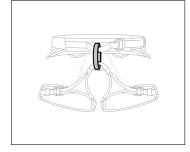
• Verify that the screws on the gated attachment point are present and properly tightened. Verify the absence of deformation, cracks, marks, wear, corrosion.
