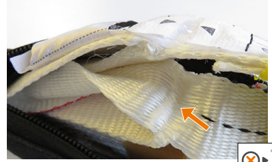
• Absorber has sustained an impact load; absorber has started to tear
