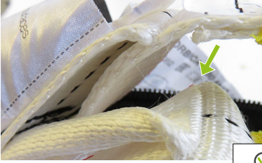
• No tearing of the energy absorber
