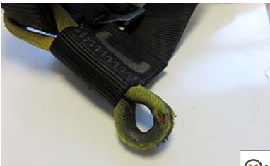
• Damaged attachment point
