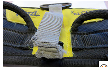
• Damaged attachment point
