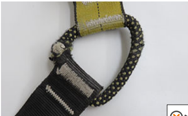
• Damaged attachment point
