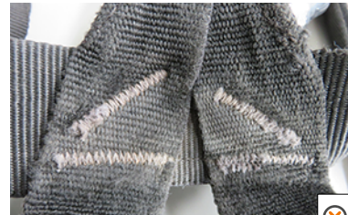
• Damaged safety stitching
