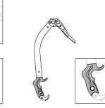
• Check the condition of the grip (marks, deformation, cracks, wear...).
