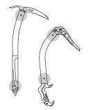
• Check the presence and condition of the rivets (marks, deformation, cracks, corrosion, absence of play...).
